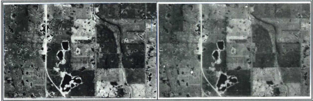
Illustration 1. The effect of haze on luminance range. The density range difference (negative) between the two conditions is .30. Film average gradient is 1.21 and the paper grade is #3.
