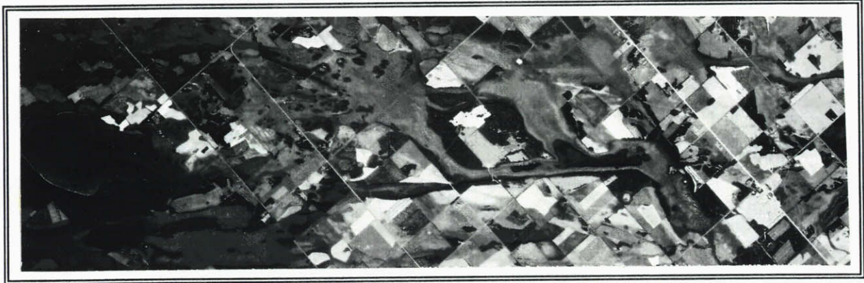
Illustration 6. 1:110 000 photography photographed with the 88 mm. lens (left is corner, right is center).
